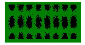
The Constellation diagram should be as focused as possible and the "dots" should be brought together as much as they can be.
