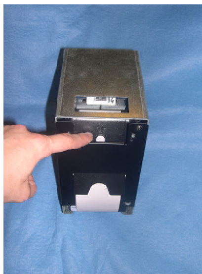
Step n°6 (you must check if you see the paper in the hole)
