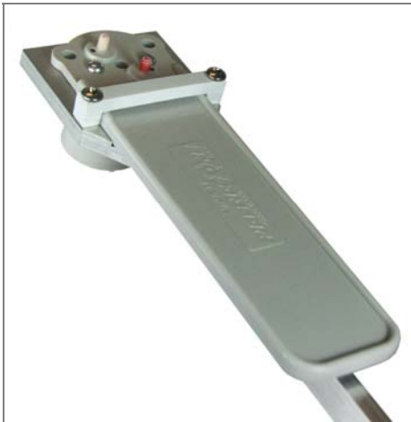
Figure 2.10 - Multi-Channel Commutator Installed on the Swivel Arm
