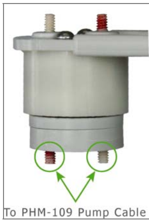
Figure 2.13 - Connect to PHM-109 Pump Cable
