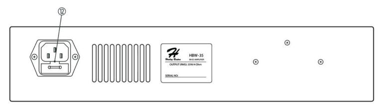
13 Panel plug for mains cable with fuse holder.
