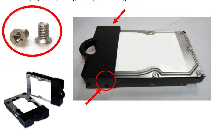
Step5: Slide HDD trays into the case.
