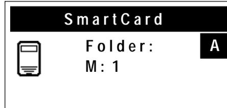
3. Rotate the Alpha dial until the desired folder appears in the display. Folders are labeled A through Z.
