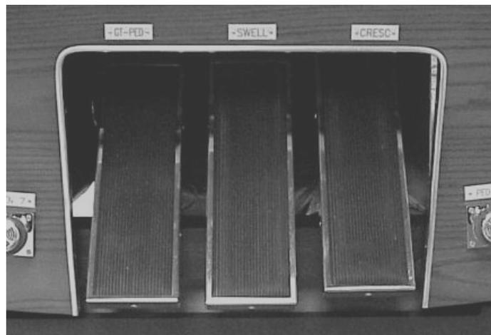
When an expression shoe is pressed forward, the volume of the division increases; when the shoe is drawn back, the volume of the division decreases. The position of the two expression shoes are displayed on two expression indicators, located on the right-hand side of the coupler rail.
