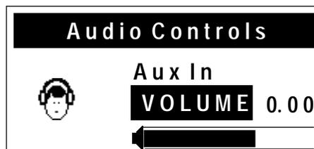
6. Rotate the Alpha dial to select the setting to be adjusted (**VOLUME, BALANCE, BASS, TREBLE**).
