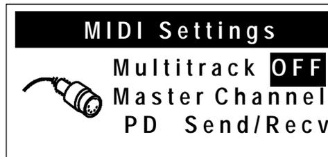
6. Rotate the Alpha dial to select the desired setting (**On** or **Off**).
