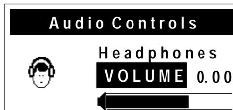
7. Rotate the Alpha dial to select the setting to be adjusted (**VOLUME, BALANCE, BASS, TREBLE**).
