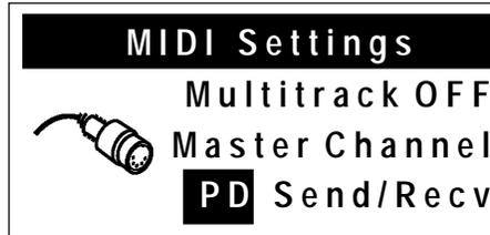
6. To change the Master Channel in the display, use the Select knob to highlight the Master Channel field (**PD** in the example above) then rotate the Alpha dial to change the selection.
