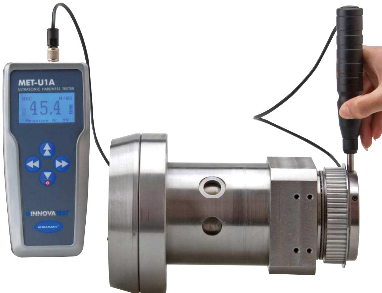
MET-U1A ULTRASONIC HARDNESS TESTER, 15N TESTFORCE
