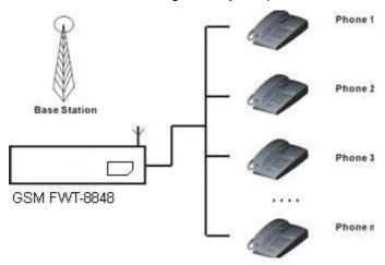
**Draw your attention:** Because there are many types of ordinary telephone and their electric parameters are different. In order to avoid mutual disturbance between telephone and terminal and affect voice quality. The distance between telephone and terminal is 1.5m at least.
