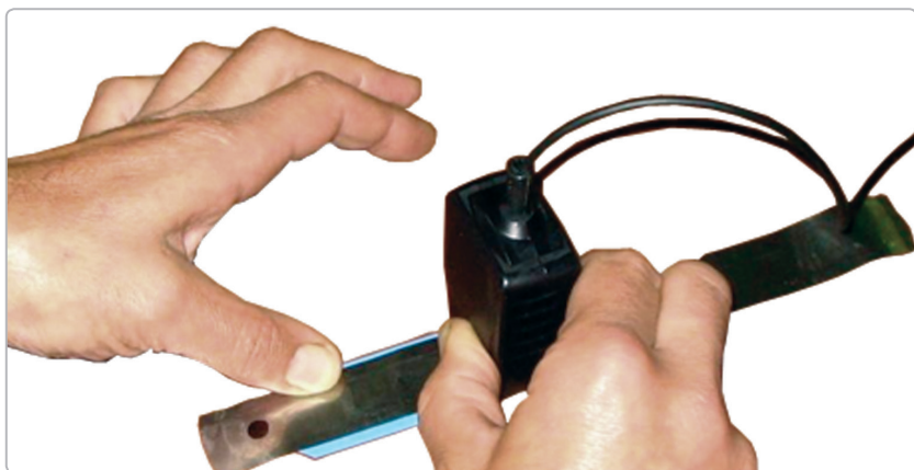
b) - magnetographing, scanner movement from left to right
