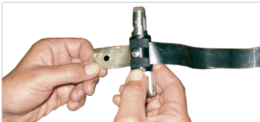
a) demagnetization, demagnetizer movement from left to right
