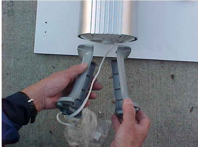
2. Tighten columns, then fix the columns with fan body by using the four screws (B).
