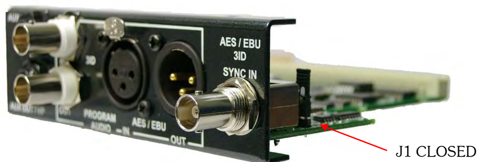
Figure 8: Terminated Sync Jumper Configuration
