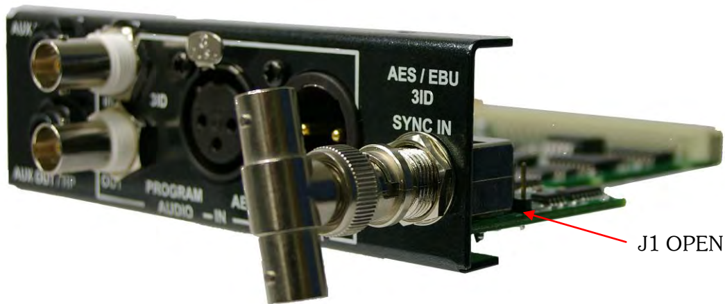
Figure 9: Unterminated Sync Jumper Configuration
