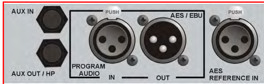
Figure 10: AES/EBU In/Out/Sync via XLR Connectors
