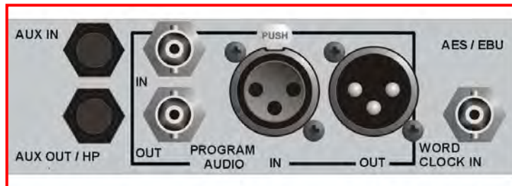
Figure 18: AES/EBU XLR and 3ID In/Out with 3ID Sync
