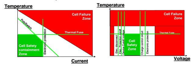
Excessive temperatures will cause cell failure. Inspired Energy batteries feature devices which will prevent further charge or discharge if exposed to high temperatures. The first level of protection devices will re-set when the temperature is lowered. There is also a thermal fuse, which will permanently shut down the battery if it is exposed to excessive temperatures.
