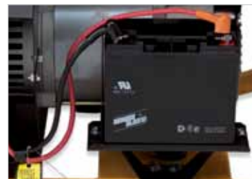
Rechargeable sealed battery—standard for electric start.
