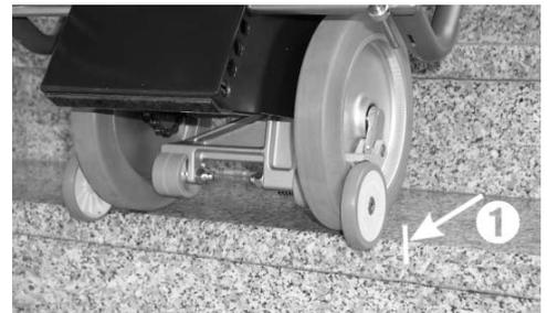
The sensitive rolls **2** of the safety brakes **3** keep the s-max from rolling over the edge.
