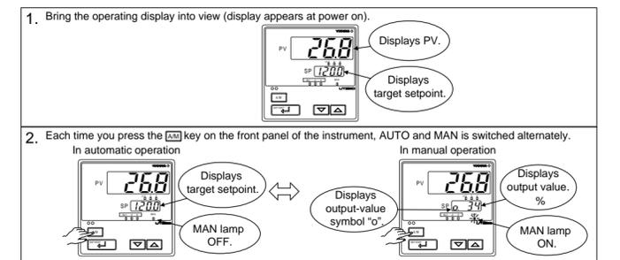
**8. Manipulating the Control Output in Manual Operation**
