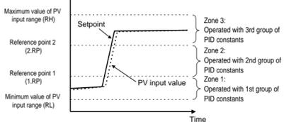
Note: Set the maximum and minimum values, as close as possible to those of the actual range to be controlled, in the Maximum Value of PV Input Range (RH) and Minimum Value of PV Input Range (RL) parameters. Otherwise, the controller may fail to determine the optimum values when auto-tuning is carried out.
