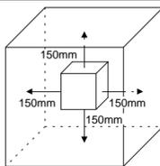
Never place the controller directly on flammable items or equipment. If the controller has to be installed close to flammable items or equipment, be sure to provide shielding panels all around the controller, at least 150mm away from every side; the panels should be made of either 1.43mm-thick metal-plated steel plates or 1.6mm-thick uncoated steel plates.
