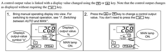
**Manipulating the Control Output during Heating/Cooling Control**
