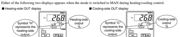
**Controller behavior and control output manipulation when the dead band is positive**
