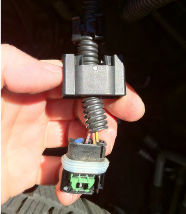
Picture 15 – Top view of the pin layout with pin1 cap removed and yellow cable ready to be installed
