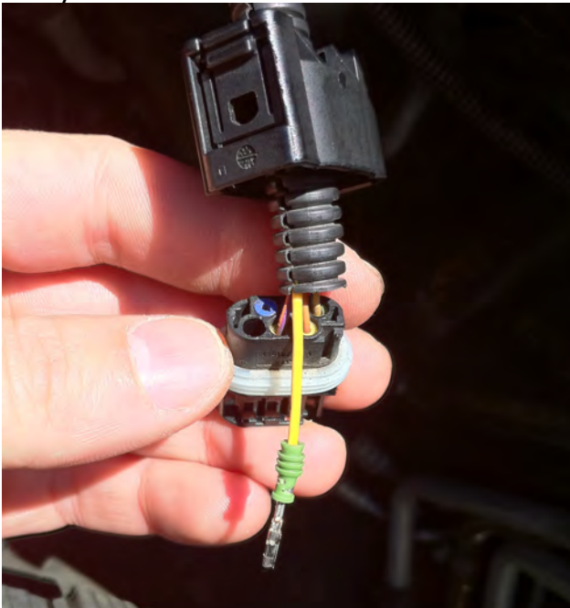
Picture 15 – Top view of the pin layout with pin1 cap removed and yellow cable ready to be installed
