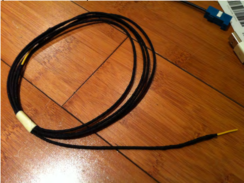
Picture 7 - Extension yellow cable – one side goes to PIN1 of aux. heater harness the other side connects to yellow cable from Telearstart module harness (shown in Picture 5 )
