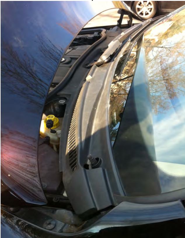
Picture 22 – After wiper arm and fuse cover replaced
