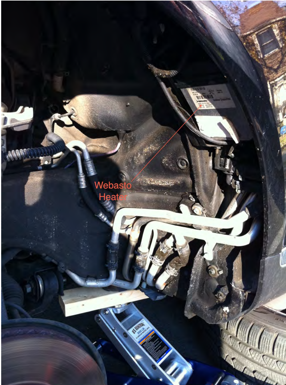
Picture 12 – Webasto heater under driver’s side front fender
