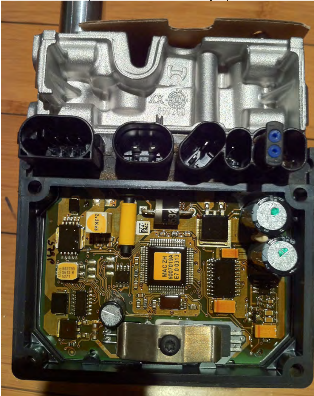
Picture 32 – The replaced old circuit board with jumper in slot 5
