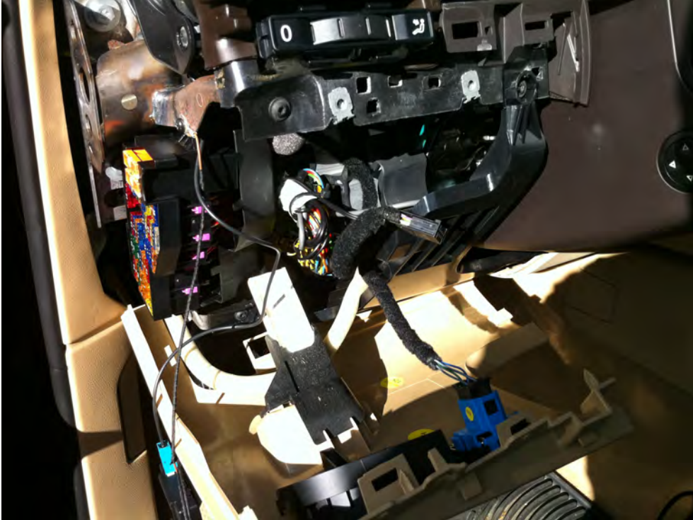
Picture 23 – left fusebox side with plastics and covers removed
