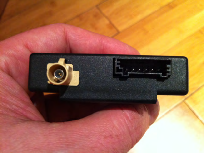
Picture 8 - Telestart module side view – antenna connector on the left and male connector for the harness on the right
