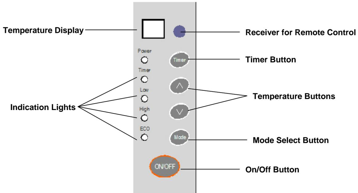
1. Turn the heater on by pressing the On/Off button on the control panel or the supplied remote control.
