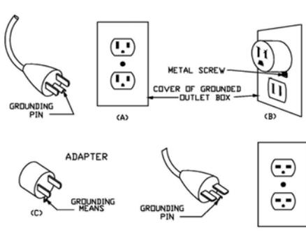
**WARNING:** This heater has a voltage rating of 120 volts. The cord has a plug as shown in A. An adapter as shown in C is available for connecting three-blade grounding-type plugs to two-slot receptacles. The grounding lug extending from the adapter must be connected to a permanent ground such as a properly grounded outlet box. The adapter should not be used if a three-slot grounded receptacle is available.
