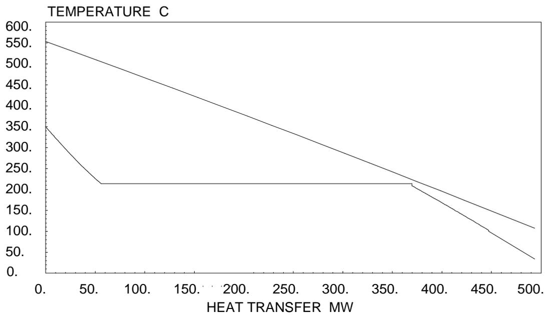
**Figure 3** TQ-diagram for the single pressure steam cycle
