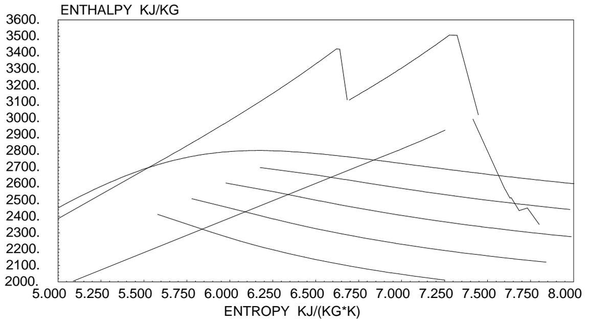
**Figure 10** *HS-diagram for the dual pressure reheat steam cycle*
