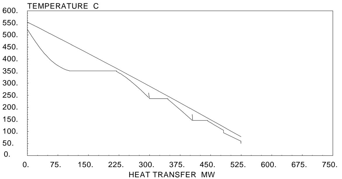
**Figure 15** TQ-diagram for the triple pressure steam cycle
