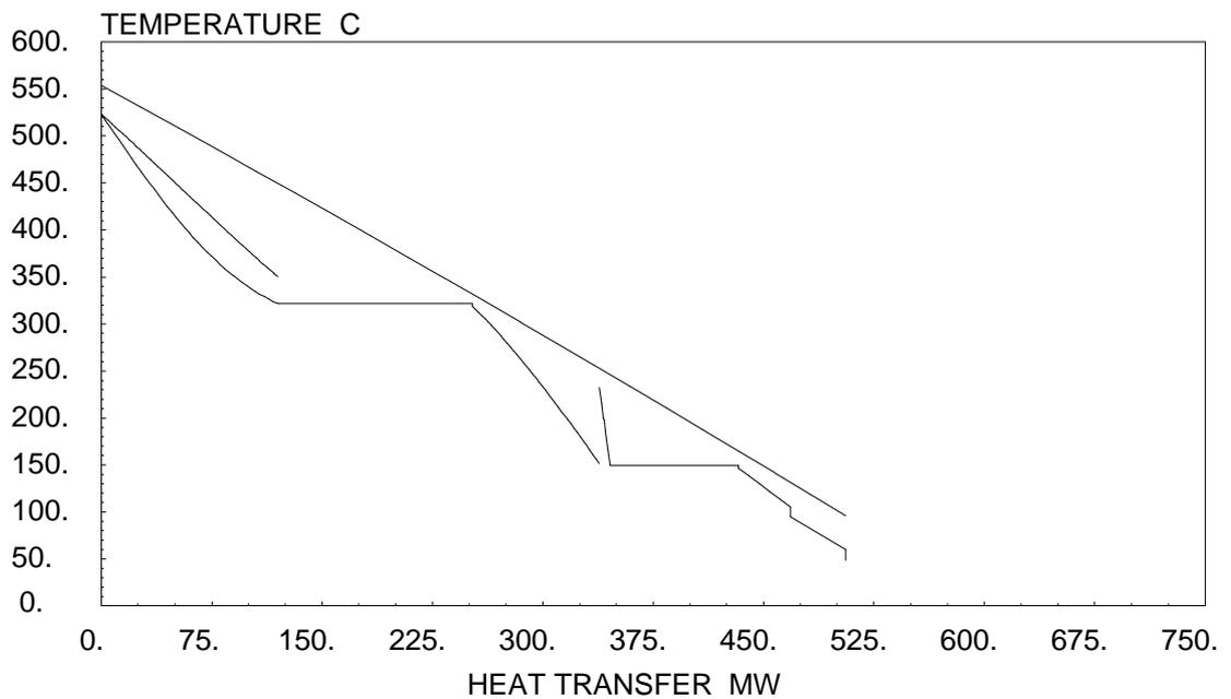
**Figure 9** TQ-diagram for the dual pressure reheat steam cycle
