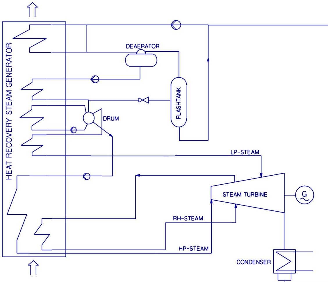
**Figure 11** Flowsheet diagram for the dual pressure supercritical reheat steam cycle
