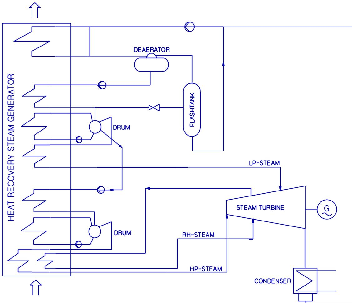
**Figure 8** Flowsheet diagram for the dual pressure reheat steam cycle
