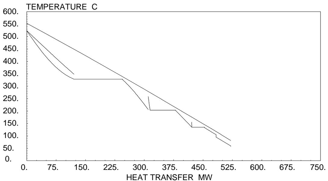
**Figure 18** TQ-diagram for the triple pressure reheat steam cycle
