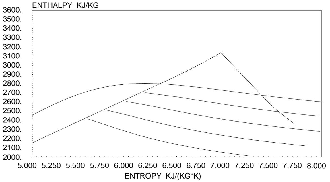
**Figure 4** *HS-diagram for the single pressure steam cycle*
