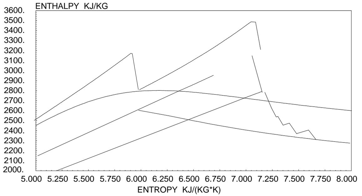
**Figure 22** *HS-diagram for the triple pressure supercritical reheat steam cycle*
