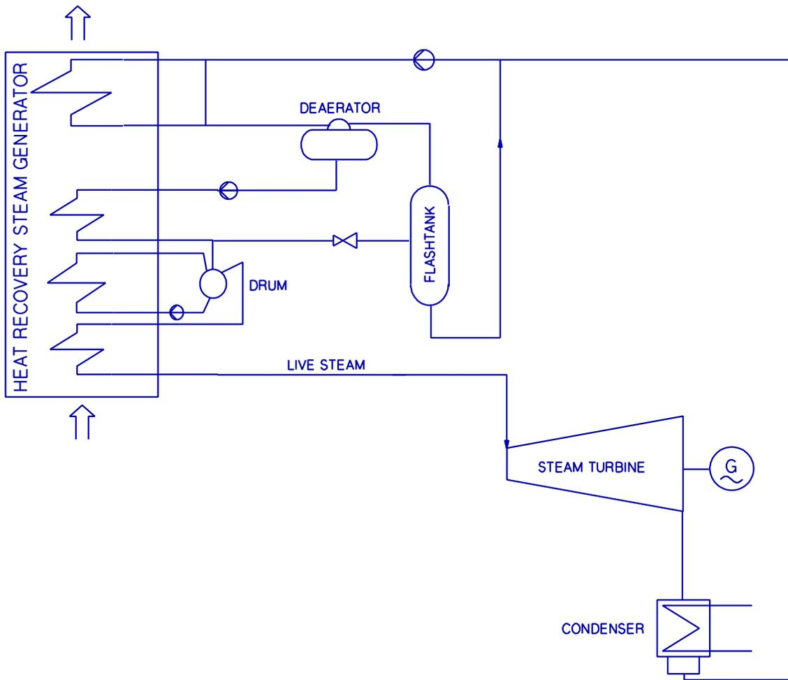
**Figure 2** Flowsheet diagram for the single pressure steam cycle
