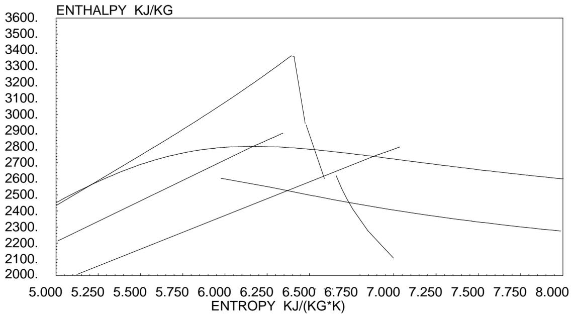
**Figure 16** *HS-diagram for the dual triple pressure steam cycle*
