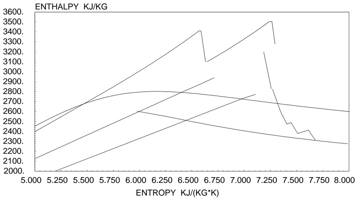
**Figure 19** *HS-diagram for the triple pressure reheat steam cycle*
