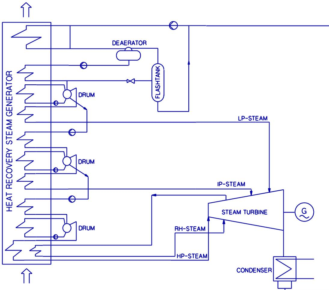
**Figure 17** Flowsheet diagram for the triple pressure reheat steam cycle
