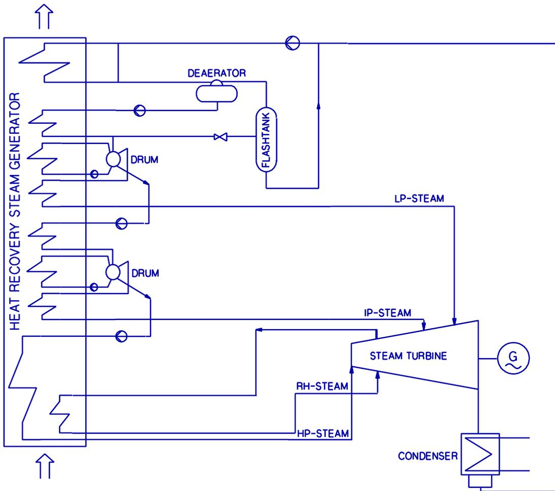
**Figure 20** Flowsheet diagram for the triple pressure supercritical reheat steam cycle
