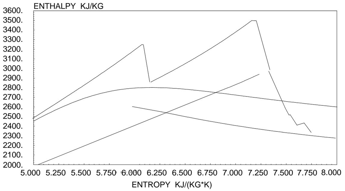
**Figure 13** *HS-diagram for the dual pressure supercritical reheat steam cycle*
