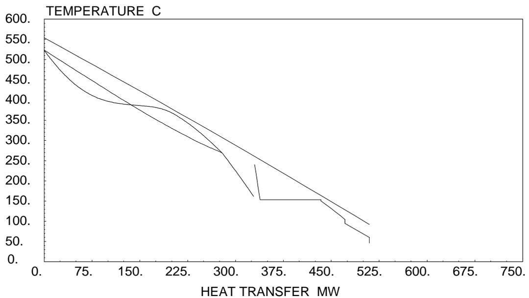
**Figure 12** TQ-diagram for the dual pressure supercritical reheat steam cycle
