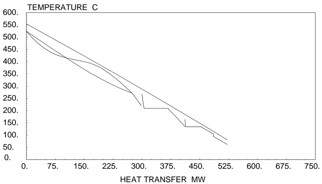
**Figure 21** TQ-diagram for the triple pressure supercritical reheat steam cycle
