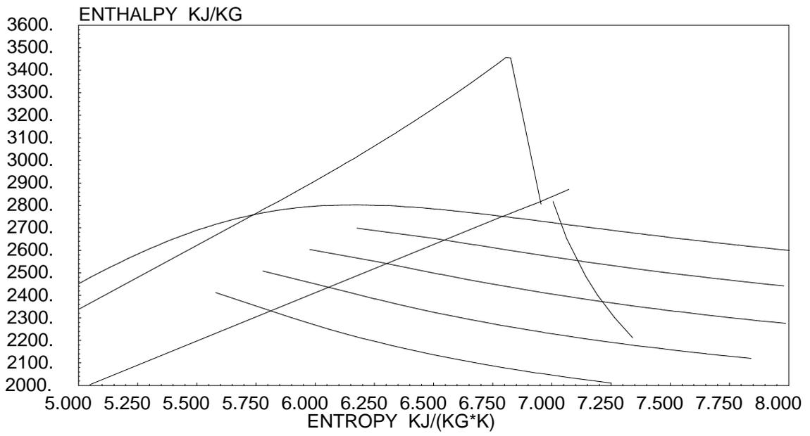
**Figure 7** *HS-diagram for the dual pressure steam cycle*
