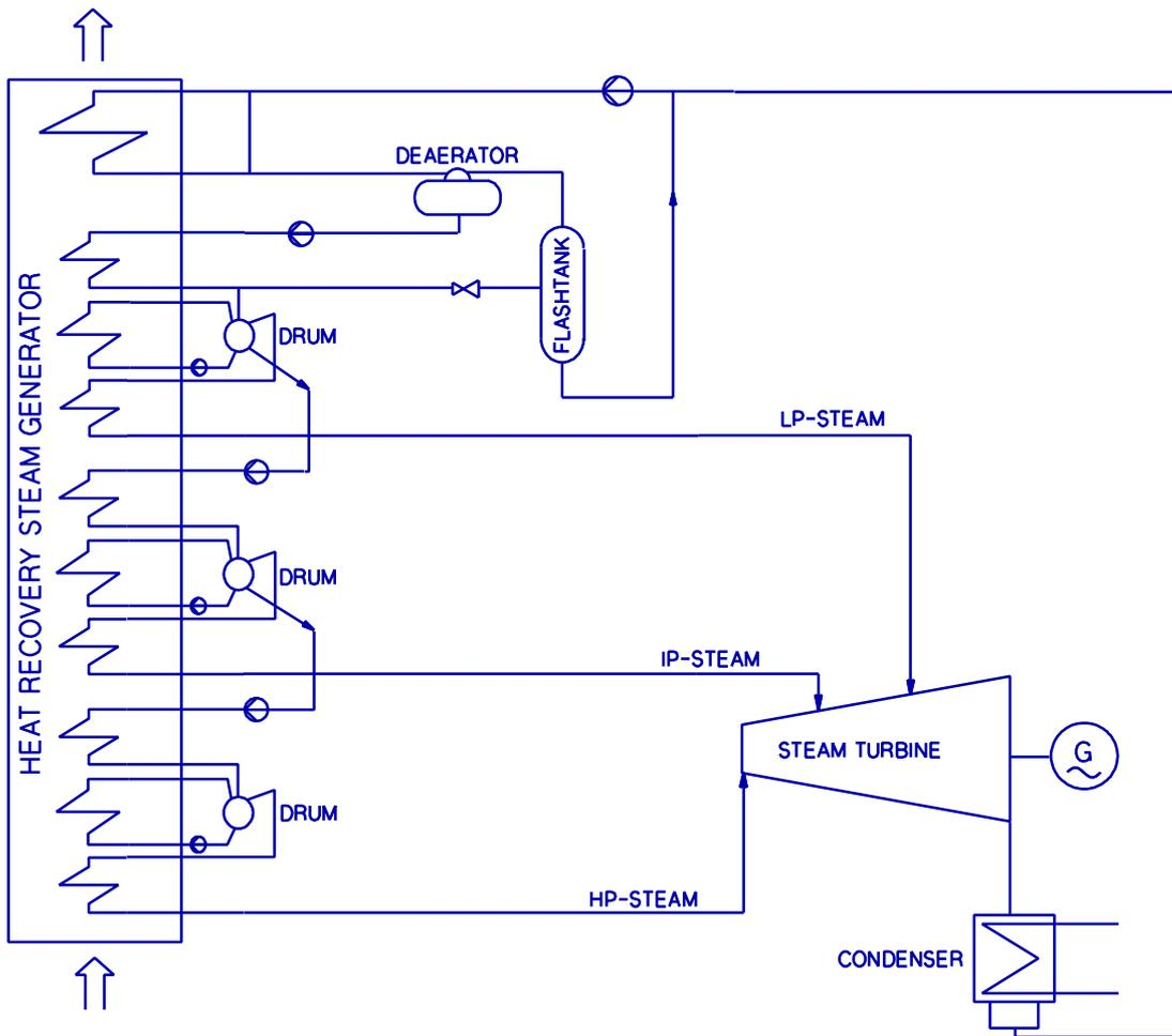
**Figure 14** Flowsheet diagram for the triple pressure steam cycle
