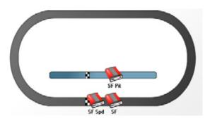
Timing and scoring with a multiloop system can add great value to a race, due to the multiple loops installed. Much more information will be available, like split times, speeds and differential times at various parts of the circuit. This is called a **Multiloop system**.
