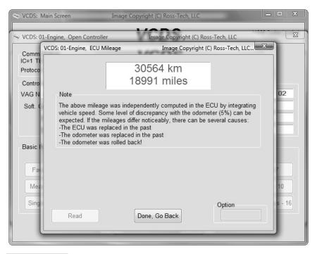
**[EDC-15 Mileage]** is found in the Applications Screen and is used to show an independent "odometer" reading stored in the ECU. EDC-15 is found in some 2000 and newer engines but is NOT used in US-market Mk4 PD engines nor is it used in the newest vehicles that use CAN-Bus diagnostics like the Mk5 Jetta TDI. This can be useful as a means of crosschecking the mileage on a used car before making a purchase, particularly in Europe where odometer fraud is rampant.
