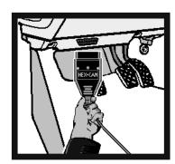
◀ If your vehicle has a 2x2 port (some pre-1996 vehicles), then use the optional 2x2 Adapter between the Interface and the ports in the car. This is included in the Pro-Kit.
