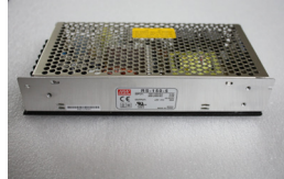
4) Power Supply: The silver box that the 110v power cable is attached to. This unit supplies all power to the components in the sign.
