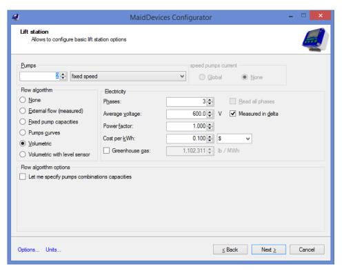
Flow algorithm selects how the flow is calculated. If the RT is not used for flow calculation, select None.
