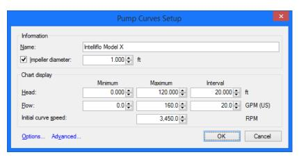
To create pump curves, enter the minimum and maximum values for the X-axis (flow) and Y (head) from the pump curve graph (like on the previous page) and the value of the intervals in the appropriate fields. Set a speed at which the first curve will be created in the **Initial curve speed** field. Start by the highest RPM curve.
