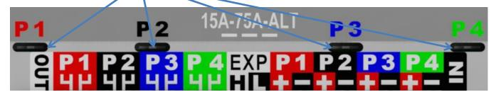
If mini current sensors (MLCT75) are used for pumps of less than 40 HP, then the DIP switch should be centered. If the size of the pumps is above 40 HP or if the inputs are used for generic analog inputs, then the DIP switches should be place to their most right position.
