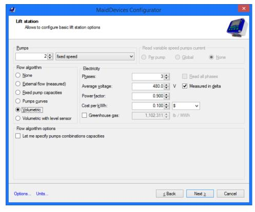
outflow is affected by the head (which is affected by the level and the force main pressure). If any of these two elements are missing, the real time accuracy will be lower.
