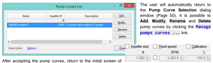
the **Pump Curves Selection**. These are advanced impeller settings and only used when the impeller may be worn or not the original impeller do to maintenance requirements. The setting will compensate for the impeller size, speed or calibration. These adjustments will only affect the system curve and not the pump curve you may have loaded into the software. On the right, you can enter the true diameter of the impeller.
