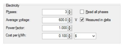
The **Electricity** section allows you to enter parameters used to calculate the power consumption of the pumps. The values are specific to the electrical configuration of each station. They are also dependent on the number and type of pumps used. The estimation of kilowatts consumed by a pump is the result of Current x Voltage x Power Factor.
