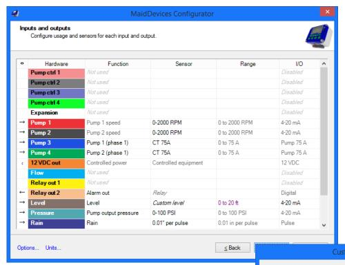
Current clamps are used to monitor the states of the pumps and their current. The input must be set to their right value by clicking on the sensor's displayed value. With fixed speed pumps, the input number represents the Pumps number. With variable speed pumps, the input number is right for the RPM monitoring, but not the current sensors as you see on the dialog on the right.
