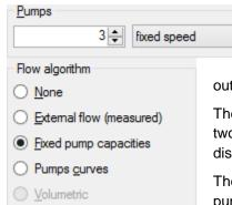
In the **Lift station** dialog window, when all pumps are constant speed, the flow algorithm will use the preset pump capacities. Based on run times for each pump, the total volumes per pump and total volumes pumped (all pumps) will be calculated as
