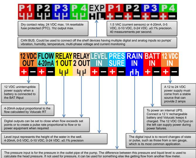
calculate the head pressure. If not used for pressure, it can be used for something else like getting flow from another flow meter. or 4-20mA, 0-5 VDC, 0-10 VDC, 0-24 VDC. ±0.1% precision
