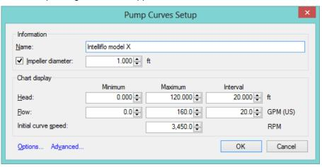
When the diameter of the impeller is known, it can be entered as part of the curve. If a different impeller diameter is used and entered in the Pump Curve Selection dialog (previous page), then the calculate flow will be automatically adjusted according to updated data on the impeller's diameter.
