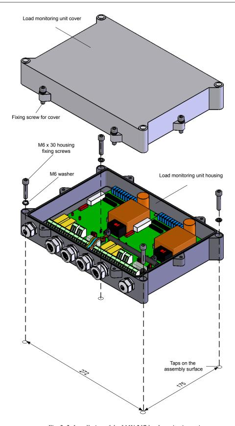
Fig. 2–2 Installation of the LMU 217 load monitoring unit
