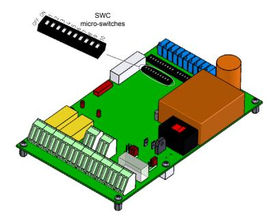
Fig. 2-12 Location of the SWC micro-switches on the load monitoring unit board
