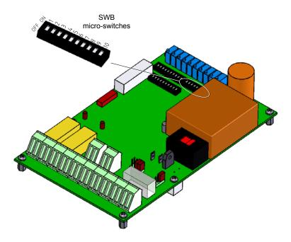
Fig. 2-11 Location of the SWB micro-switches on the load monitoring unit board
