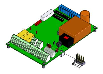
Fig. 2-13 Location of the transducer presence simulation jumpers
