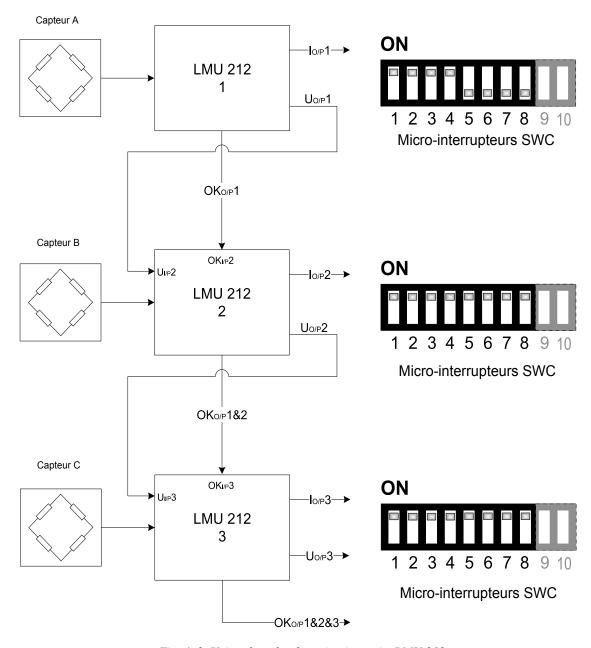
Fig. 4–3 Using three load monitoring units LMU 212
