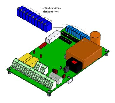
Fig. 2-10 Potentiometer location on the load monitoring unit board
