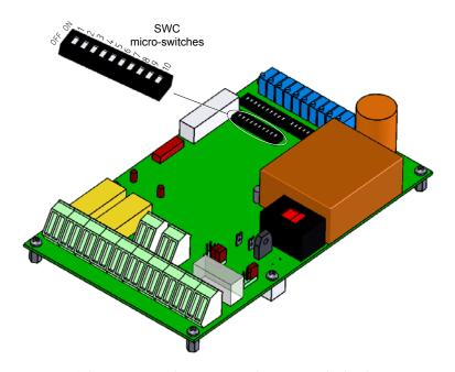
Fig. 3-2 Location of the micro-switches SWC3 and SWC4 on the load monitoring unit board
