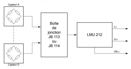
Fig. 4–4 Using one single load monitoring unit LMU 212
