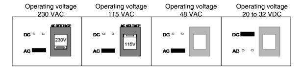
Fig. 2–5 Jumper and switch configuration
