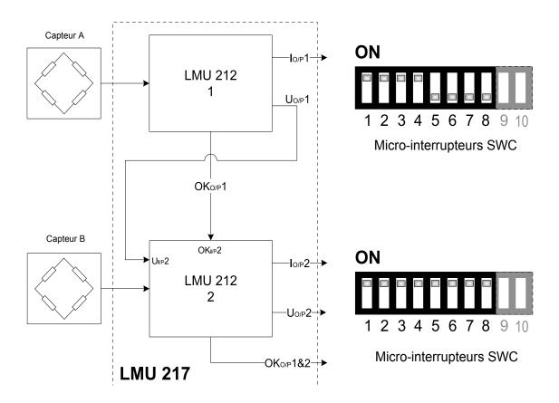
Fig. 4–2 Using one single load monitoring unit LMU 217
