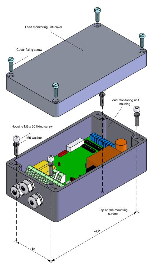
Fig. 2–1 Installation of the LMU 212 load monitoring unit
