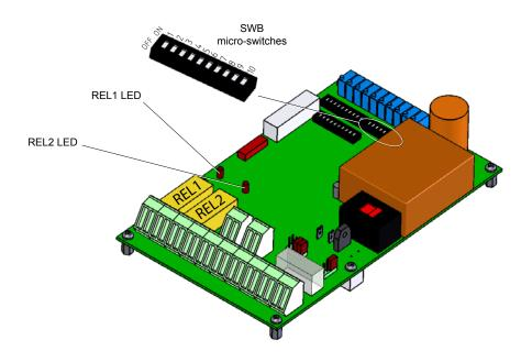
Fig. 3-3 Location of the relays REL1 and REL2 on the load monitoring unit board
