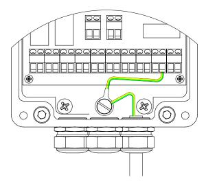
Fig. 2-6 LMU grounding when using a 230, 115 or 48 VAC supply
