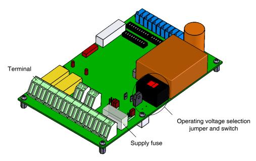
Fig. 2-4 Load monitoring unit board with location of the selection elements
