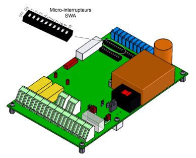
Fig. 2–8 Location of the SWA micro-switches
