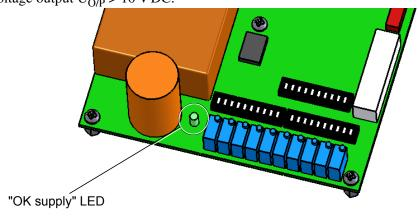
Fig. 4–5 Permanent supply check LED
