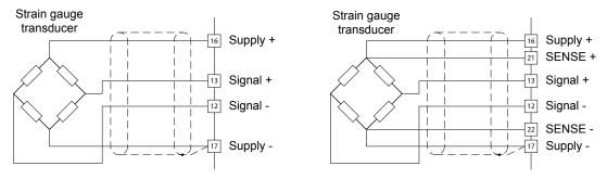
Fig. 2-7 Wiring types
