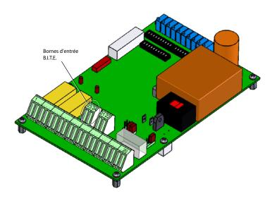
Fig. 4-6 B.I.T.E. control input terminals
