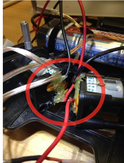
Figure 17. - Motors with Capacitors
