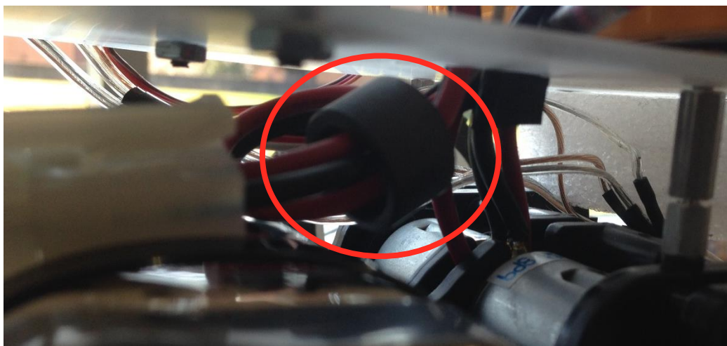
Figure 12. - Ferrite Core Choke on RC Car Battery
