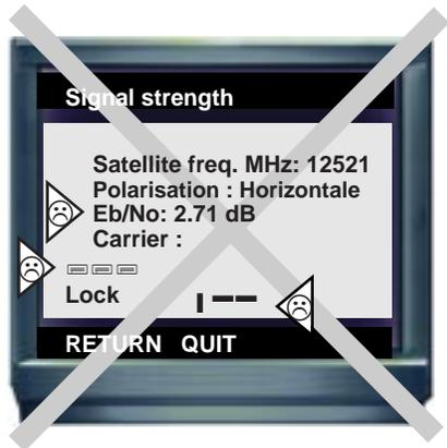
The above screen shows that the satellite reception installation is faulty or incorrectly adjusted. The three parameters "Carrier", "Lockout" and Eb/No show a reception malfunction.
