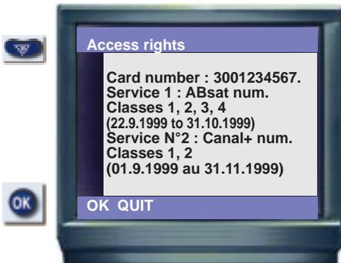
→ This screen, accessed via MENU and then SMART CARD, is used to modify some parameters included in the access card. It is possible to modify the card's "access level" in particular (see relevant paragraph). The same screen is used to modify the Secret Code and to consult the current access rights (subscriptions). Choose INFORMATION and then enter the prememorized Secret Code (32896)+, to check the current subscription rights of your card.
