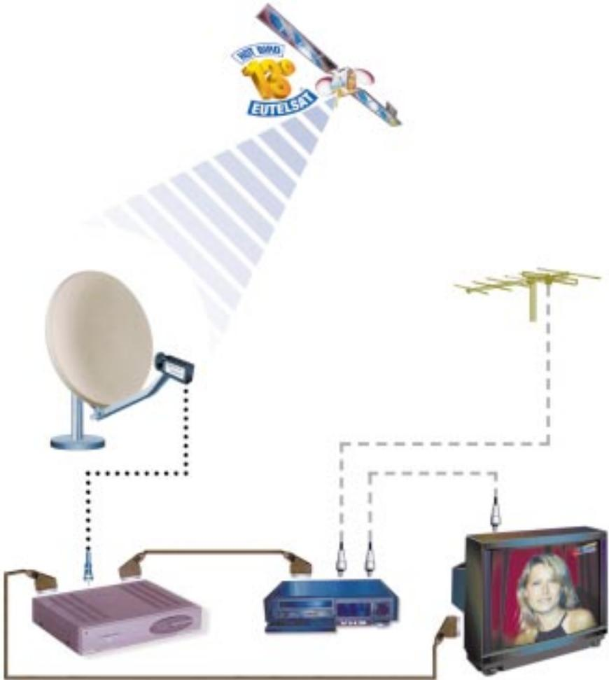
For DiSEqC compatible LNBs and DiSEqC adaptors, ask your reseller or your antenna technician: the XSAT CD.TV350 receiver uses the Level 1.1 DiSEqC standard.
