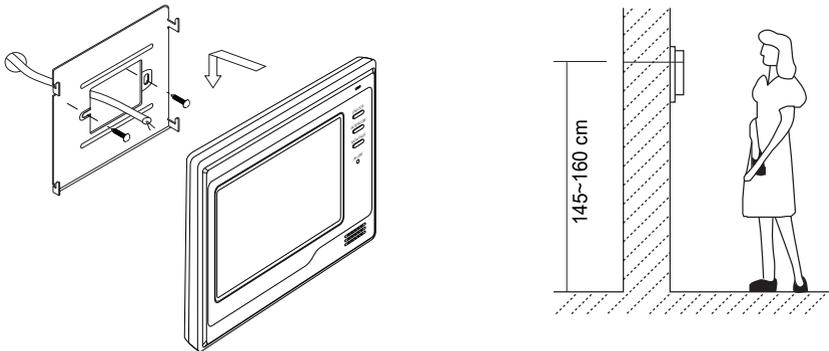
1. Use the screws to fix the Mounting Bracket on the mounting box.(fitting accessories includes a Bracket (Two pieces of 4X25 screws are needed for fastening the Mounting Bracket), Special 2 wire cables to connect with Monitor)
