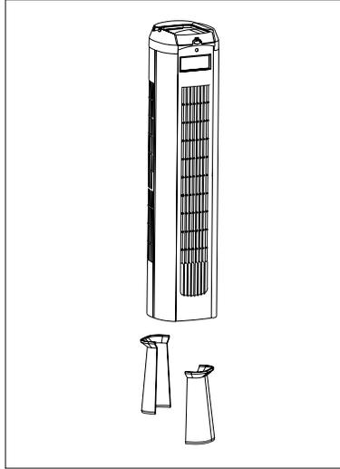
3. Attach the fan base to the pedestal. Like the pedestal, the fan base is made up of two separate halves. Make sure the power cord passes through the middle of the fan base. There is a groove on the bottom of the fan base for the power cord. Make sure this groove is aligned with the back of the fan prior to securing the fan base to the pedestal.
