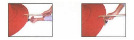
The wore cutters can be change easily with a cutter dismantle spanner. It must be lifted up to cutter fix pin gets free when the cutters dismantled. When mantle of new cutters, be careful to be cutting side is bottom.
