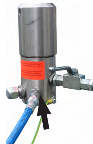
Fig. 30: Connecting spraying hose to high pressure filter
