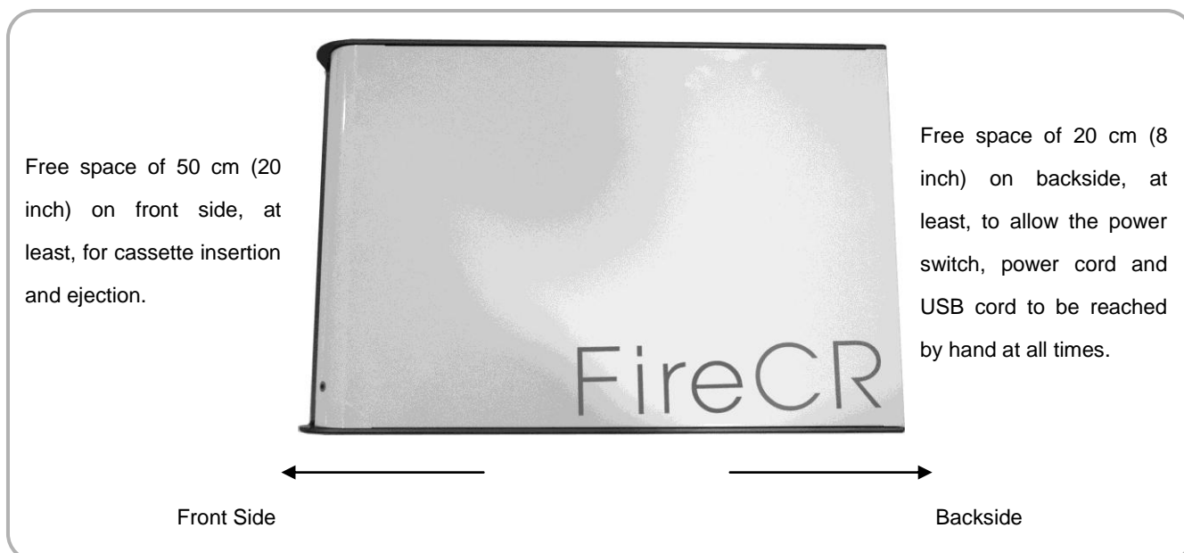
Figure 4. Tabletop Mount Space Requirements (Top View)
