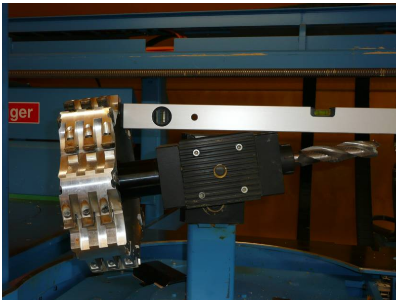
Picture – Bevel UM = Deviation from the horizontal position
