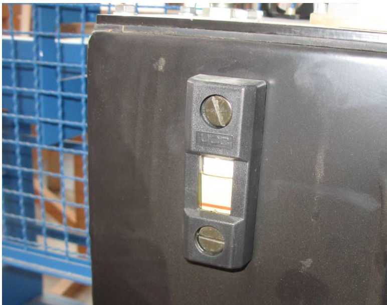
Picture – Hydraulic aggregate: The oil level must be within the upper 30% mark.
