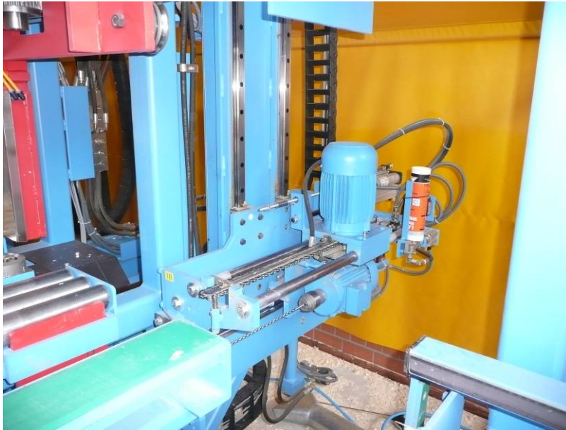
Picture – Drill and Slot cutter create the “movable combi-support”
