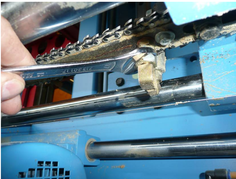
Picture – The cartridge with the chain lubricant is connected with a pipe to the chain guide
