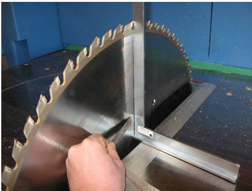
Picture – Checking the position of the saw blade in relation to the machine table
