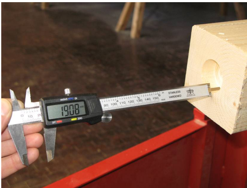
Picture – measured depth approximately 19 mm
