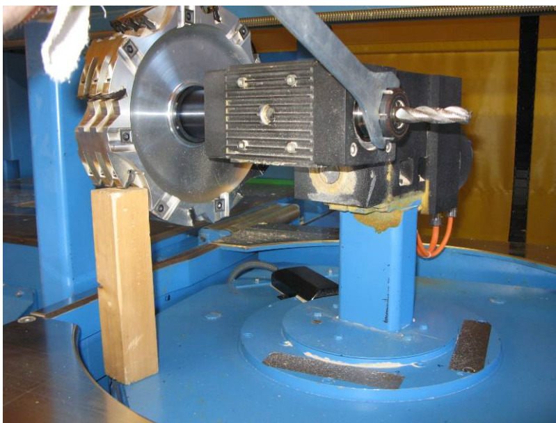
Picture – unscrew the 20 mm end mill
