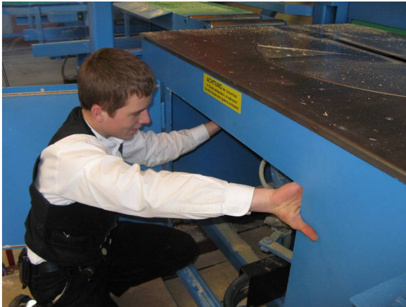
Picture – Right hand pushes the release button, left hand moves the saw left and again right
