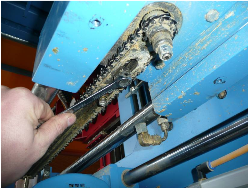
Picture – Machine from below. The screw is being loosened, SW 13
