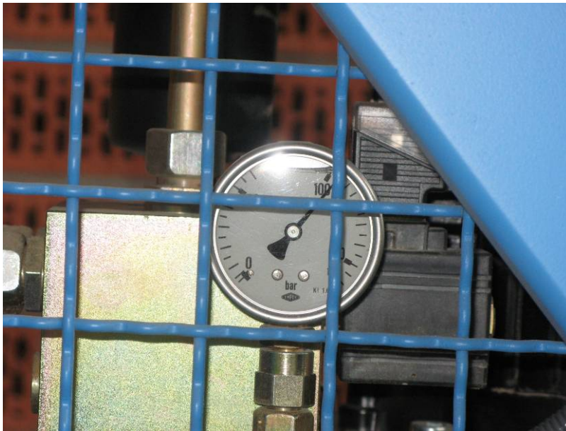
Picture – Gauge glass (pressure during full load – 100 bar)
