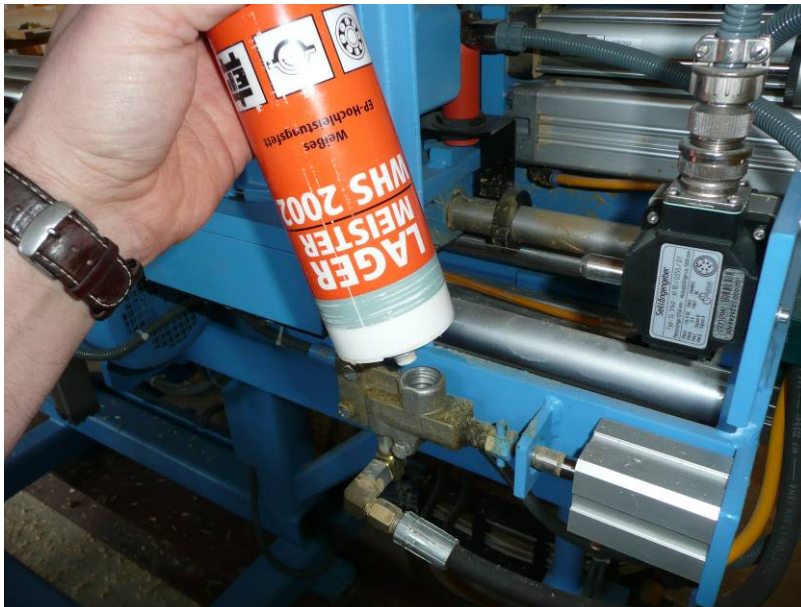
Picture – Exchange of the cartridge
