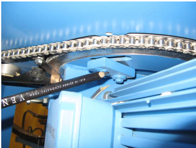
Picture – Adjust the tightness of the rolls
