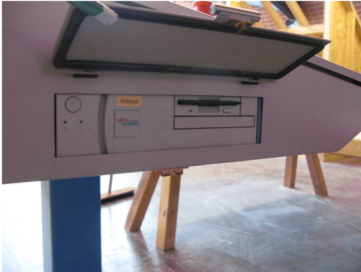
Picture – The data can be transferred via the disk drive on the side of the machine, via the network or by using USB sticks.
