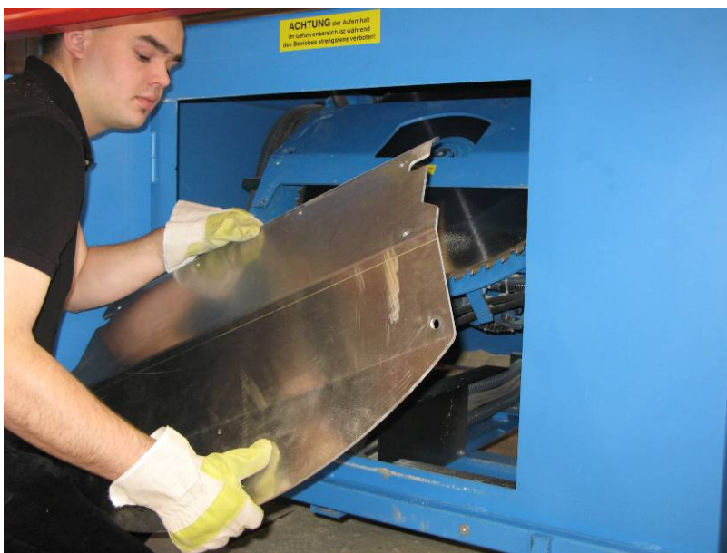
Picture – Protection is being removed
