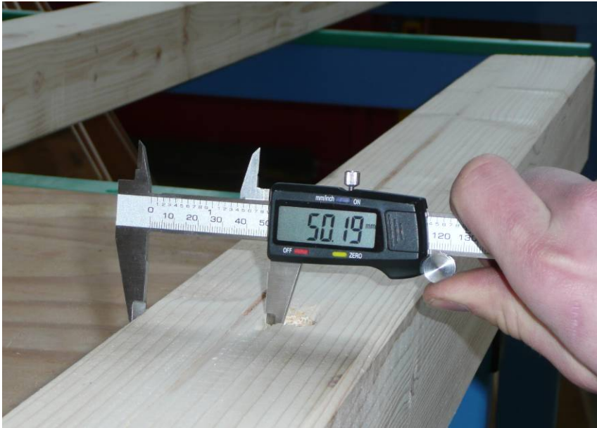
Picture – measured distance from the edge is 50.19 mm
