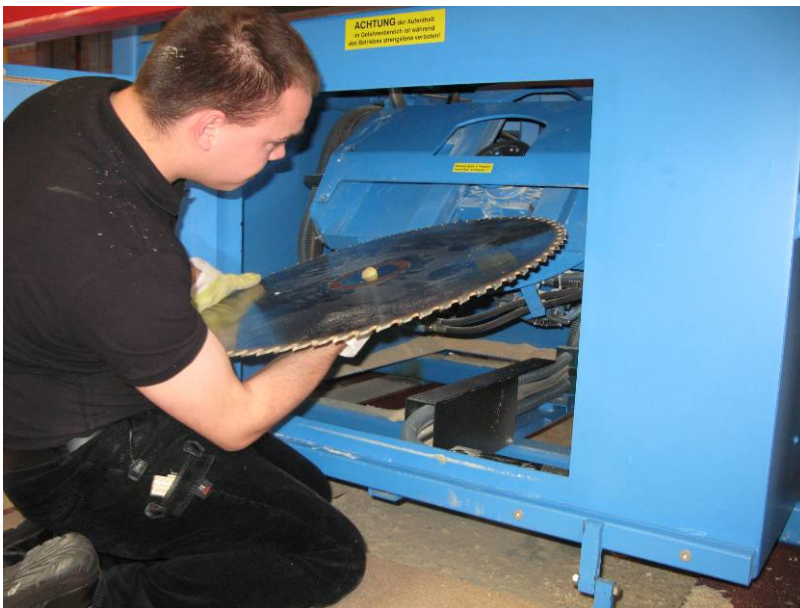
Pictures – Removal of the saw blade and visual check
