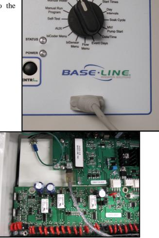
**Previous Generations of BL3200 Controllers The optional Interface** Cable is plugged into the controller board as shown – the cable should be left in place once it is installed .
