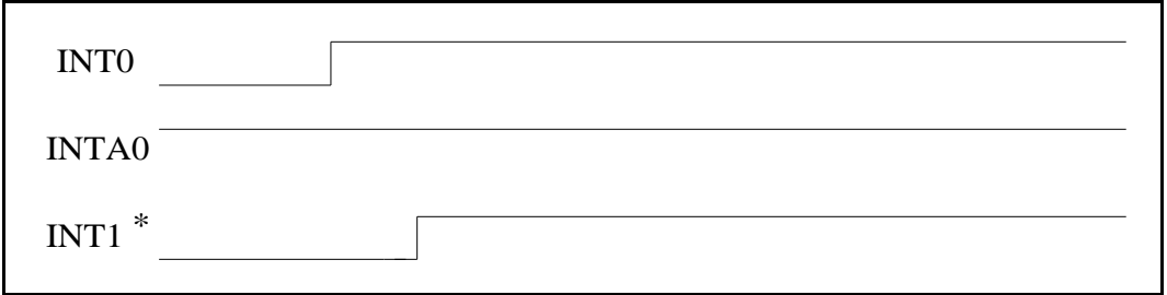
Figure 5. Incorrect INT0 Acknowledge Operation with a Simultaneous INT1
