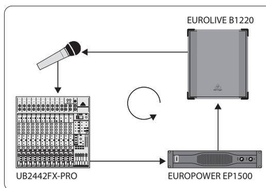
Fig. 2.1: How a feedback loop is created
