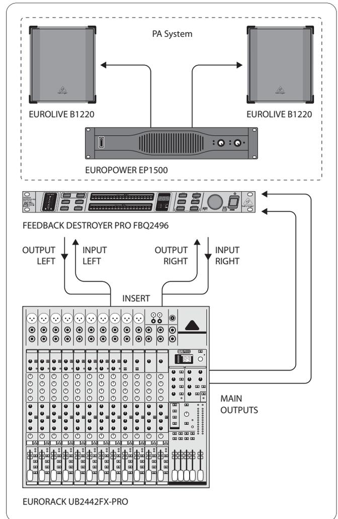
Fig. 5.2: FEEDBACK DESTROYER PRO in channel insert/subgroup insert
