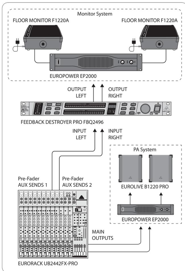
Fig. 5.1: Using the FBQ2496 in the monitor path
