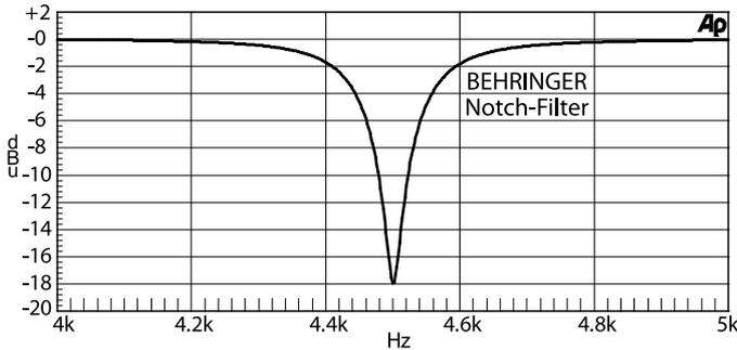
Fig. 4.1: Filter curve of a narrow-band filter
