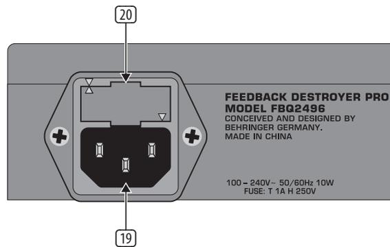
Fig.3.4: Mains connector, fuse switch and serial number
