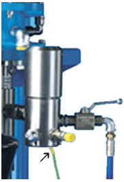
Picture 2.4.1 Grounding screw on the high-pressure filter
