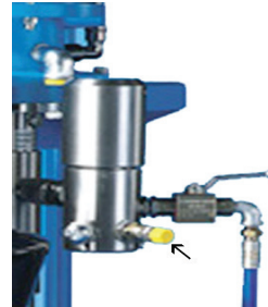
Picture 4.2 Spray hose connection on the high-pressure filter
