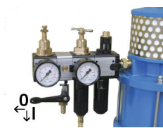
Picture 2.10.5 compressed regulator on Phoenix-Air Combi 11032
