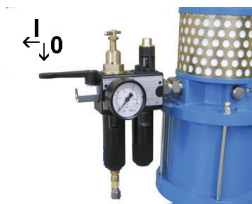
Picture 2.10.3 compressed regulator on Phoenix-Airless 6552 and 11032 and Hot Job-units
