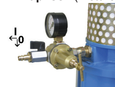
Picture 2.10.2 compressed regulator on Phoenix-Airless 6530 and 11018
