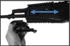
Press button on left side of gun Swing stock around Latch into place
