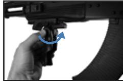
To flip hand grip up and down press the Center button in and flip handle
