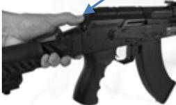
Push in the lock and remove the top cover
