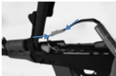
Plug battery into plug. Push the fuse back down into it's compartment.
