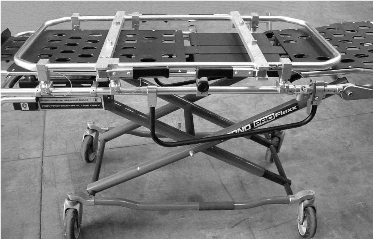
Figure 15: Installing the ITC frame on the Ferno 35P Proflexx stretcher.
