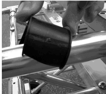
Figure 1: Assembling plastic spacers (code 2042729).
