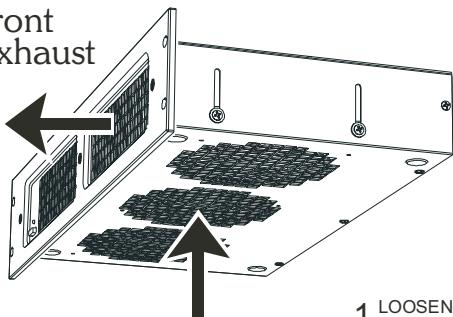
1 LOOSEN SCREWS ON BOTH SIDES AND LOWER INSIDE FAN ASSEMBLY TO BOTTOM POSITION AND RETIGHTEN
