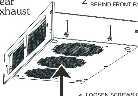
2 REMOVE TOP COVER AND PLACE FOAM BLOCK BEHIND FRONT PANEL TO BLOCK AIR FLOW
