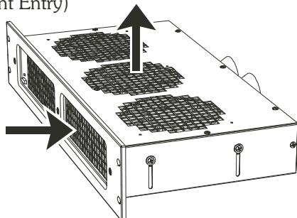
1 LOOSEN SCREWS ON BOTH SIDES AND RAISE INSIDE FAN ASSEMBLY TO TOP POSITION AND RETIGHTEN
