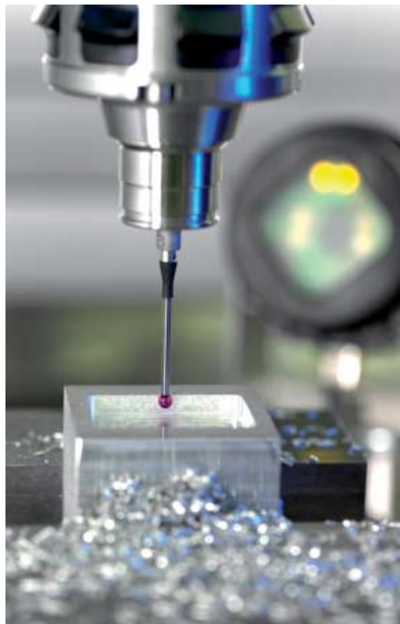
Circular pocket/hole measurement
