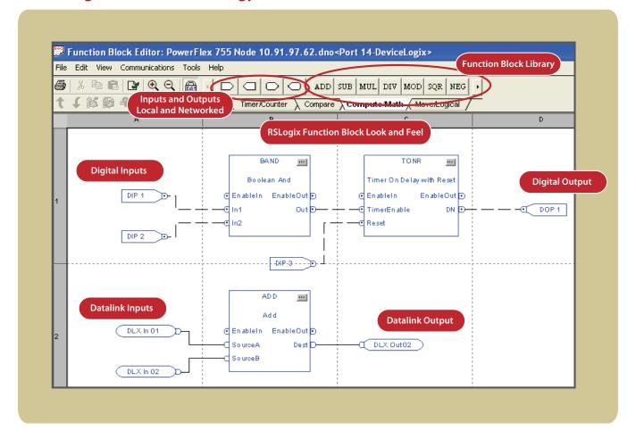
DeviceLogix control technology provides you with the flexibility to customize a drive to more closely match your application needs. DeviceLogix controls outputs and manages status information locally within the drive allowing you to operate the drive independently or complimentary to supervisory control helping to improve system performance and productivity.
