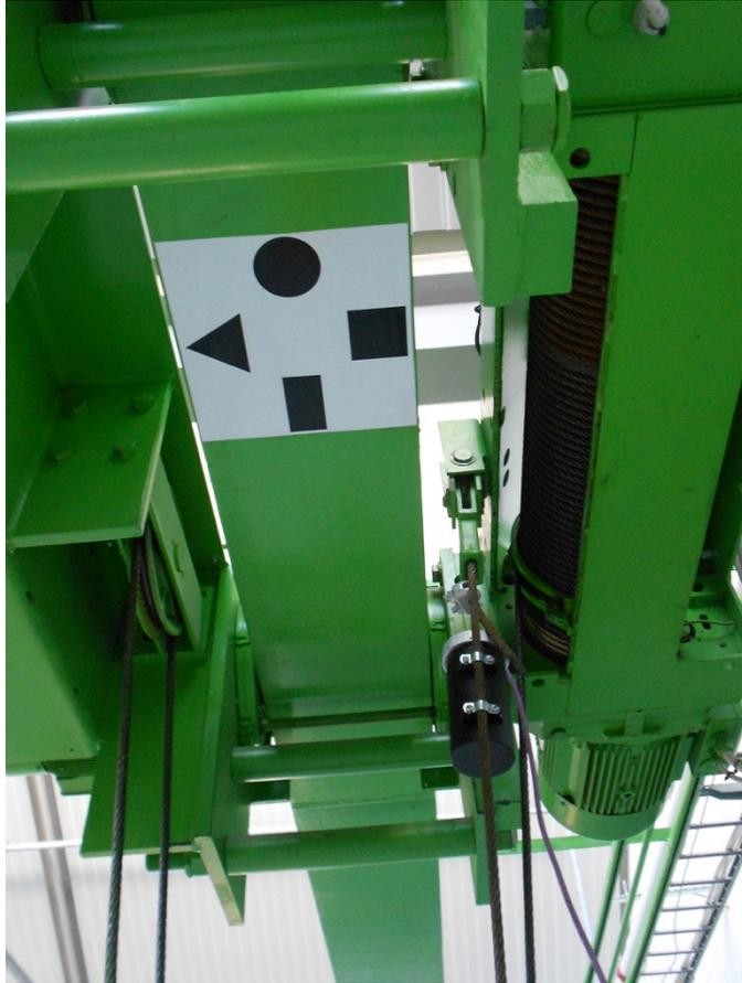
**Picture 2. Ensuring the correct installation onto the crane. Cable facing upwards, led lamp facing downwards.**
