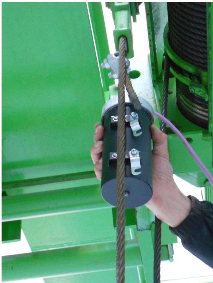
**Picture 1. Device correctly against the rope. Modbus connection cable facing upwards, led lamp facing downwards. The device is ready to be fastened.**
