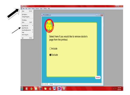
6. The following screen (a pop-up window) will appear, asking you to choose where you would like to save your data. If you want to save the data on a USB drive, insert a thumb drive into the computer's USB port. You can choose to save the data on the computer where the program is hosted but we do not recommend that option. It is recommended to save the data on a device to which selected staff only has access.
