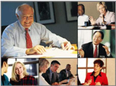
Advanced Continuous Presence Layout (5+1) - In this mode the Intelligent Call Management will use 4*CIF resolution for better clarity and H.263 video compression
