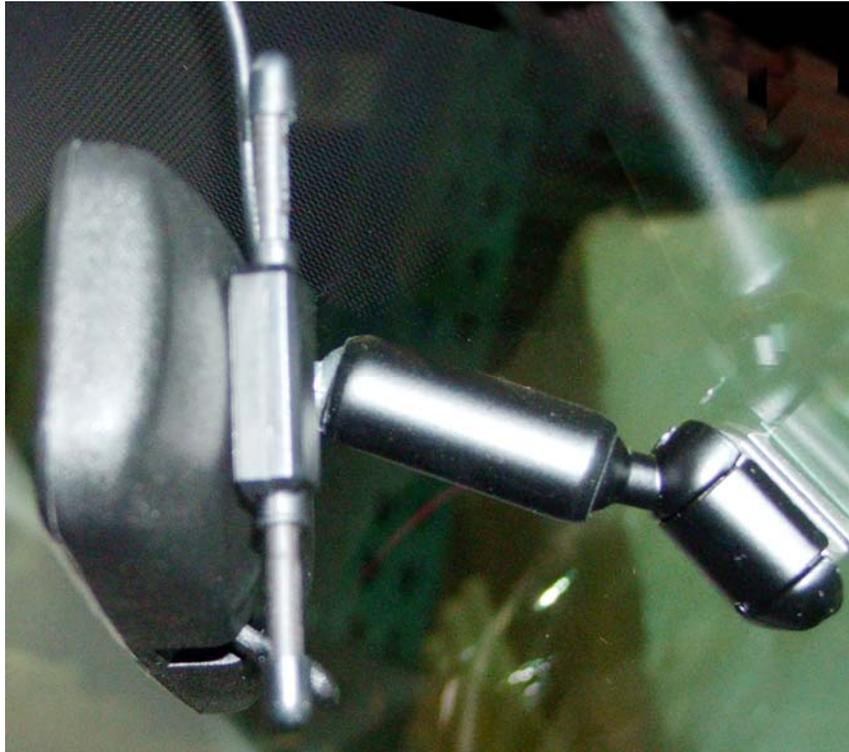
***NOTE: THIS ANTENNA REQUIRES "LINE-OF-SITE" ACCESS TO THE WINDSHIELD AND SHOULD NOT BE BLOCKED. DOING SO WILL REDUCE THE EFFECTIVE RANGE OF THIS DEVICE***
