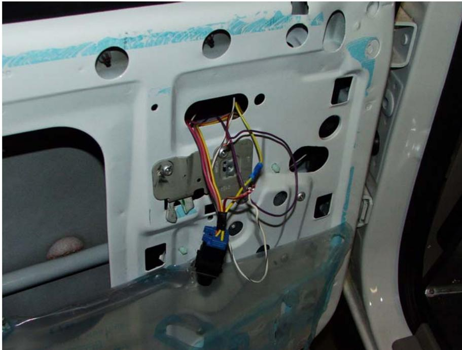
Push switch back through hole and attach to inside of door as noted below.
