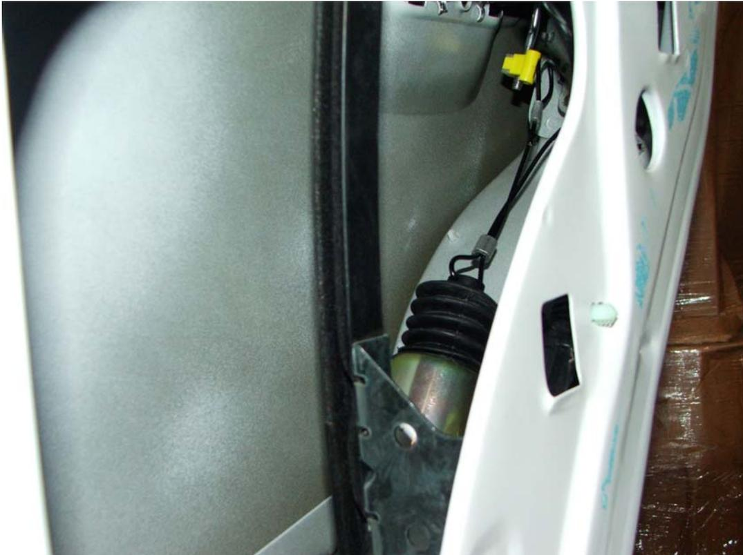
**NOTE: CABLE NEEDS TO BE ADJUSTED SO THAT DOOR LATCH IS FULLY ACTUATED WHEN SOLENOID IS COMPRESSED.**
