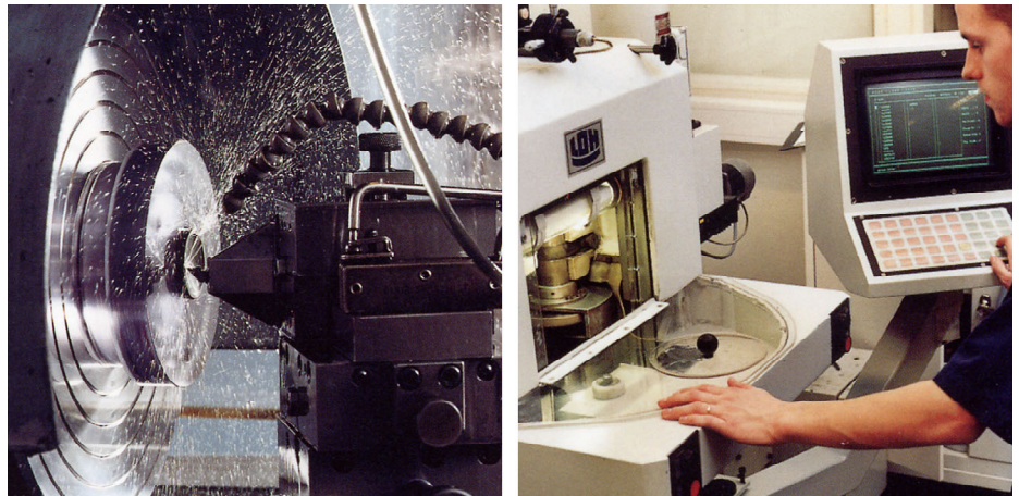
Figure 13.4 LEFT: Diamond turning machine; RIGHT: Lens polishing
