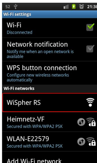
If you cannot see the WiSpher RS network, this would mean that the module has been configured for the Wi-Fi client mode. To change back to the access point mode please reset WiSpher RS to the factory settings (see chapter Restoring Factory Settings).
