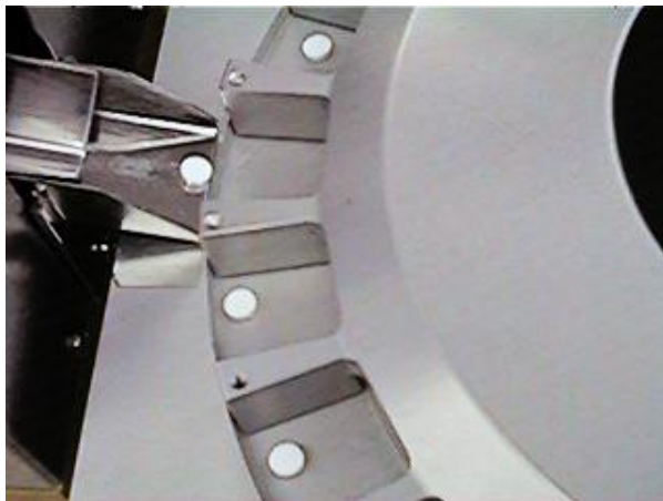
Sample transportation from the WHT-SM multiple batch feeder into WHT 3ME
