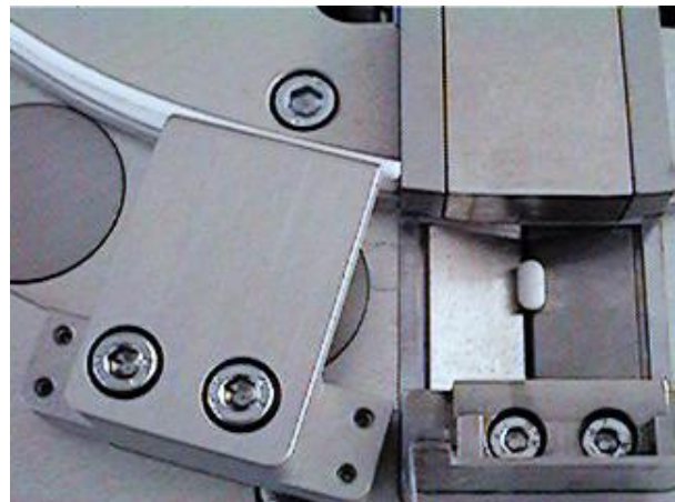
The unique feature of the WHT 3ME is the “flap” device. It positions the sample precisely in the combined diameter and hardness test station.
