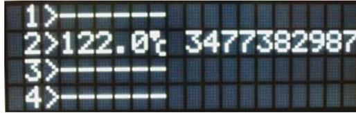
**Figure 8: Maximum memory temperature display**
