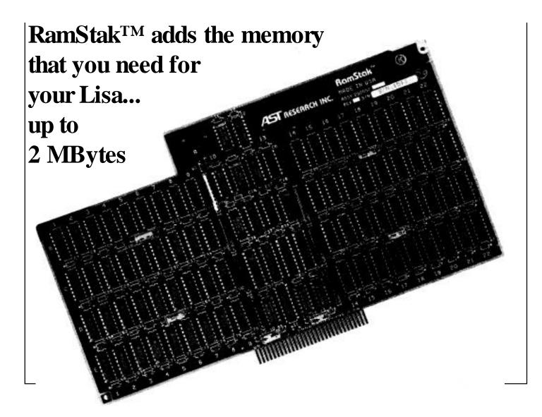
RamStak<sup>TM</sup> from AST Research is the easy plug in memory expansion board for your Lisa<sup>TM</sup> (Macintosh XL<sup>TM</sup>). The board makes it possible for professional users to configure their Lisa<sup>TM</sup> systems with up to two megaybytes of memory.
