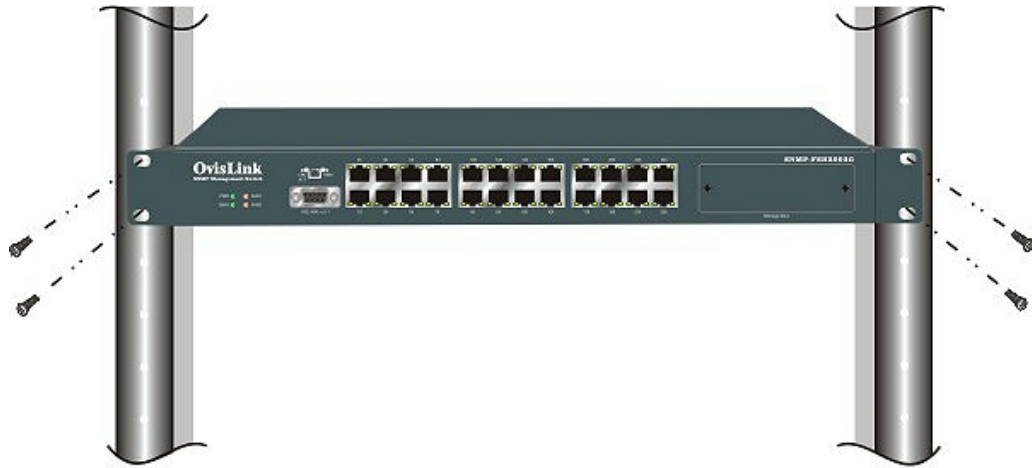
Fig. 2-5 Attaching the Switch to a 19-inch rack
